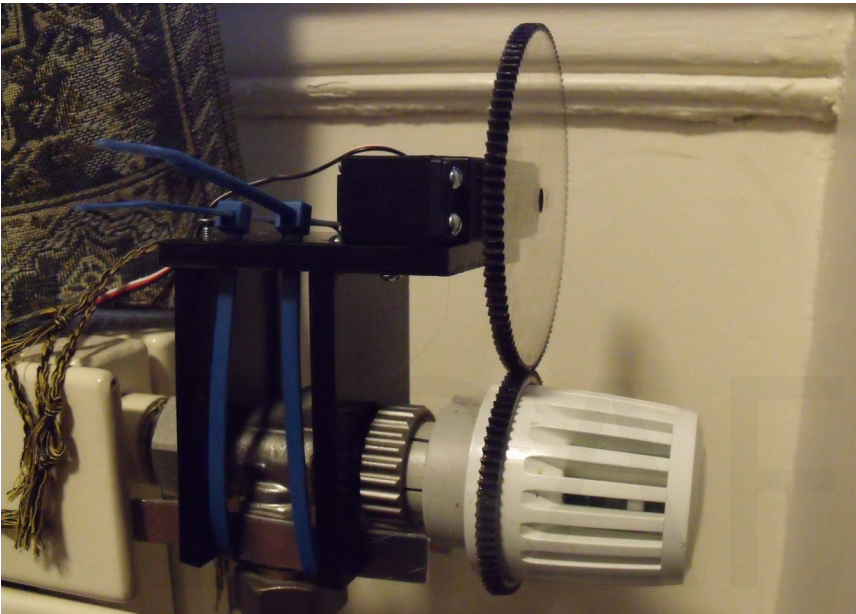
◀ The Hot Dorms team used zip ties and laser-cut gears in preliminary performance tests.
